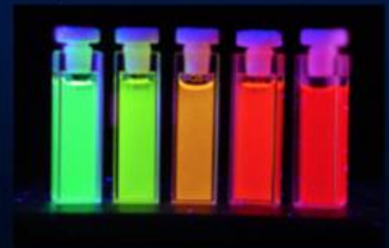
Solutions of different sized CdSe/ZnS quantum dots
