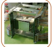
**VT:** 4 layers Si pixel (20x20 μm) **IT:** 2 layers Si pixel (20x20 μm)
