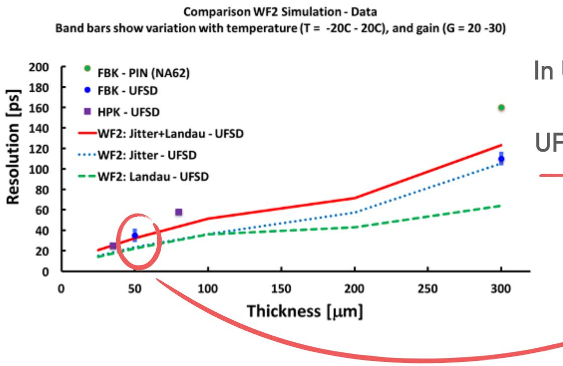
Sensors with 25 and 35 µm active thickness have been manufactured within the FBK ExFlu0 production ---- 15-20 ps resolution looks achievable with thinner sensors
