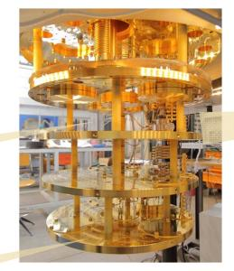
5 RF lines installed from 300 K to MixCh
