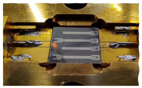
Prototype Devices fabricated at CNR-IFN with <sup>24</sup> shadow mask evaporation technique
