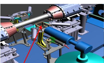
Target just behind the luminometer, which is used as trigger Charged Kaon Mass puzzle: ready for a feasibility test run using Pb target
