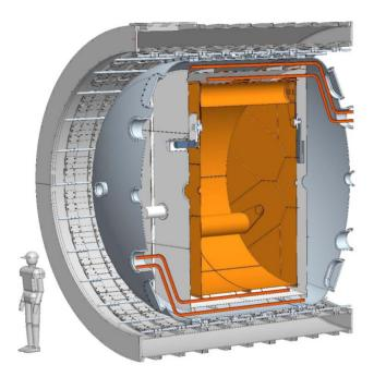
Due to their very big dimensions, KLOE or FINUDA magnets can be unique facilities to host a resonant cavity and become part of an haloscope for very low mass axions.
