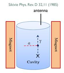
$\beta$  antenna coupling to cavity
