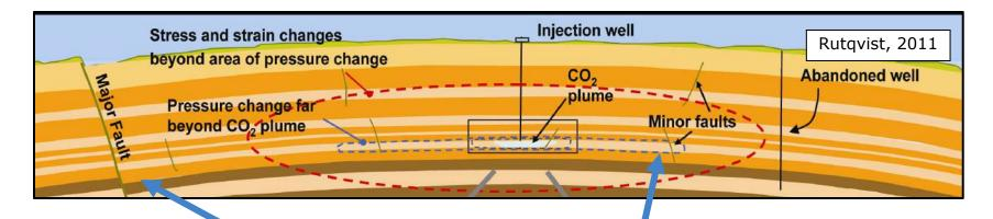
Large offset major faults can be detected at the ground surface and by seismic surveys. Sequestration site might be designed to stay away from such faults.  The regional injection-induced (slow) crustal straining and minor (hidden) faults might be of greatest concern at future large scale injection sites (minor faults of unknown location and orientation)
