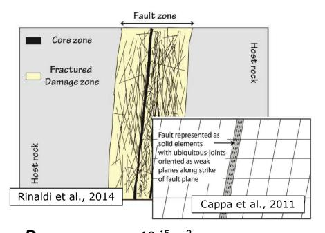
**Damage zone**:  $10^{-15} \text{ m}^2$ porosity as function of mean effective stress ( $\sigma'_M$ ), permeability depends on porosity changes (Davies and Davies, 2001)
