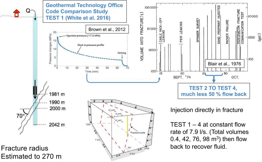
Hydroshearing model for fracture zone
