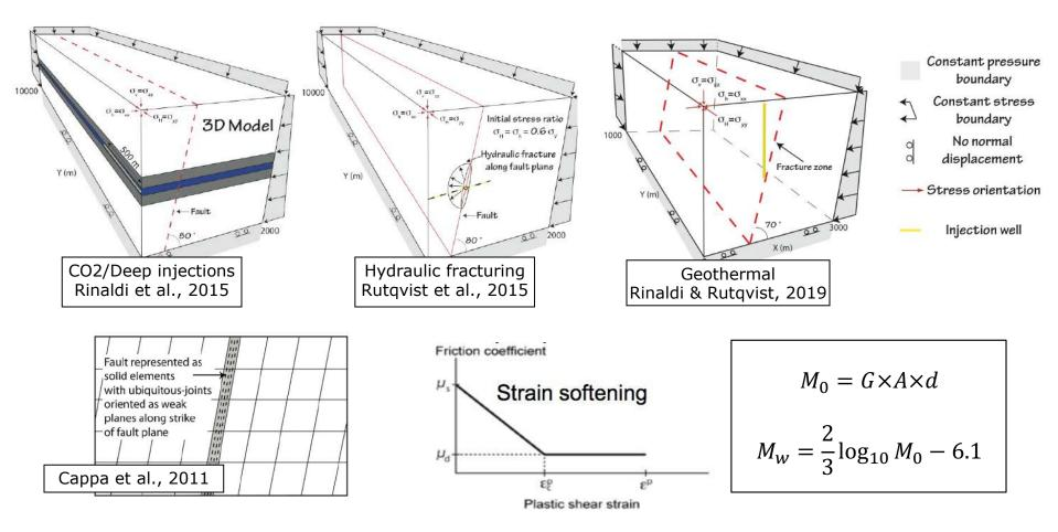
Finite continuum fault, size and permeability depending on the case
