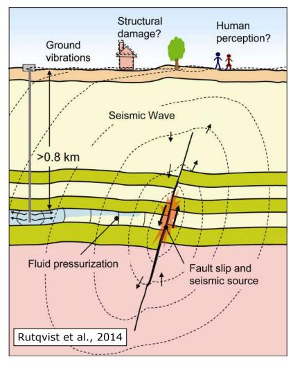
• Overpressures due to large-scale fluid injection may induce seismic events
