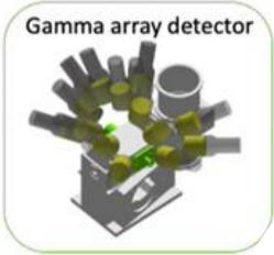
The  $\gamma$  array detector **GASTLY** has been developed and installed at CIRCE since 2018 to study nuclear reaction with charged particle in exit channel.
