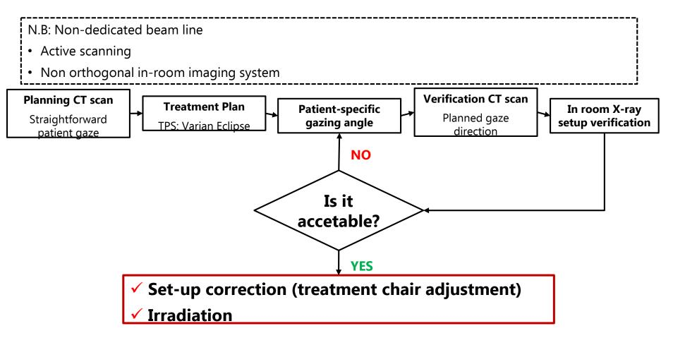
The requirement of a gaze stabilization and eye motion monitoring device during CT scans and irradiation was fulfilled by means of a compact and portable Eye Tracking System conceived for 3D real-time video oculography
