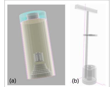
Figure 3: (a) 3D layout of the geometry reproduced in MC simulations; (b) detail of the vial holder inside the ionization chamber.
