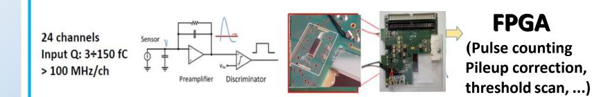
Dedicated fast ASIC chip for particle counting and readout boards (under test)
