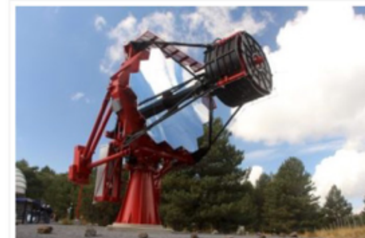
The ASTRI-Horn prototype telescope is located at the observing station of the INAF Astrophysical Observatory of Catania, in Serra La Nave, on Etna, where it was installed in 2014. The primary tassellated mirror has a diameter of 4 meters and the secondary monolithic mirror is 1.8 meters in diameter.
