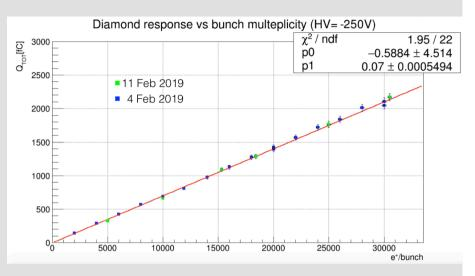
Target: collected charge vs beam multiplicity (evaluated by lead glass Cherenkov calorimeter)
