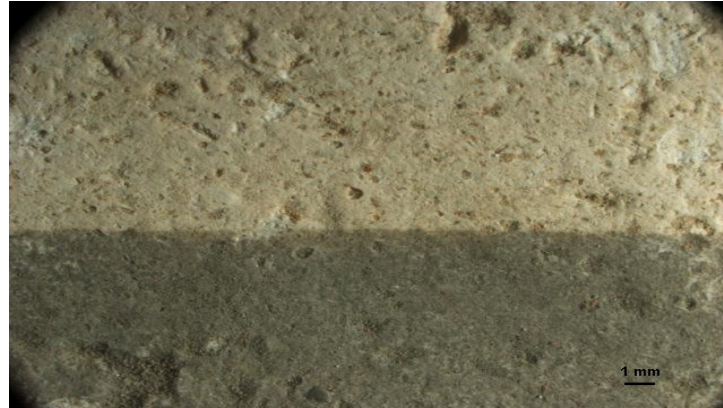
Border soiled-cleaned 475 mJ/cm 2 (bar = 1mm)
