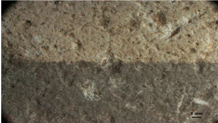
Border soiled-cleaned 450 mJ/cm 2 (bar = 1mm)
