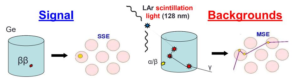
**Point-like (single-site)** energy deposition inside one HP-Ge diode
