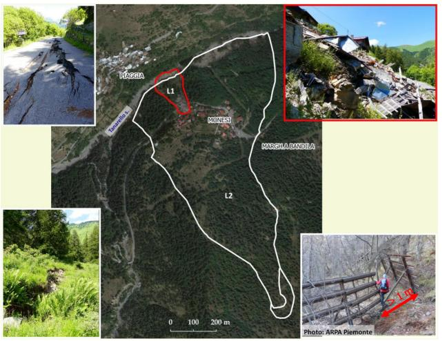
L1: Rotational landslide that collapsed destroyng road and buildings.
