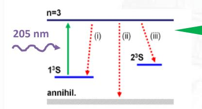
Production of metastable positronium for inertial sensing measurements
