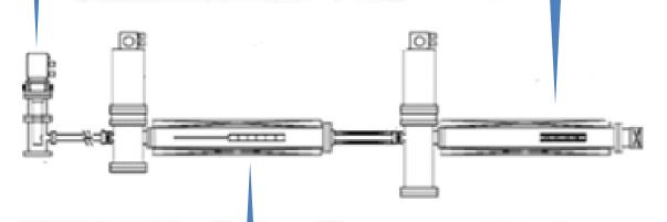
Buffer gas positron trap. Around 15% of incoming positrons are trapped in a Penning-Malmberg trap to produce bunches of up to some 10<sup>5</sup> positron/s
