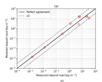
Comparison with ground measurements at 10 locations of deposit thickness and particle grain size distribution (mode)
