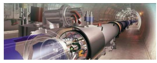
1232 superconducting dipoles 15m long at 1.9 K, B=8.33 T Inner coil diameter = 56 mm
