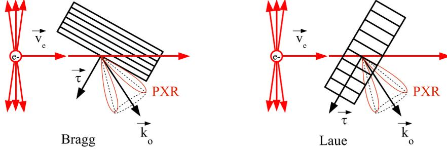
Fig. 1. – Bragg geometry (left) and Laue geometry (right) for PXR emission.
