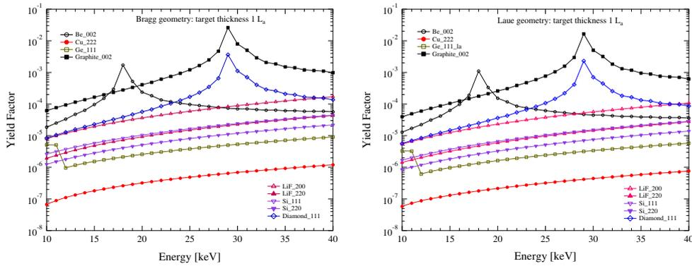
Fig. 3. – The yield factor for Bragg geometry (right) and Laue geometry (left) as a function of X-ray energy for different target crystals.
