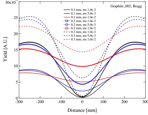
Fig. 4. – Calculation of PXR intensity profiles for different values of multiple scattering and crystal thickness.
