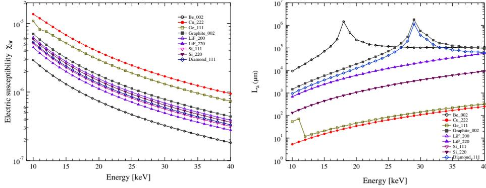
Fig. 2. – The real component of electric susceptibility  $\chi_{hr}$  (left), the geometrical factor  $f_{geo}$  (right) as a function of X-ray energy for different target crystals.
