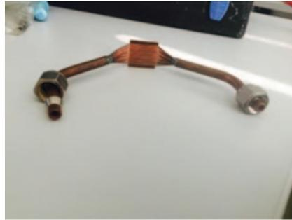
Fig. 2. – Target used for the tests. The beam impinges on the part where tubes are accommodated in the backing.
