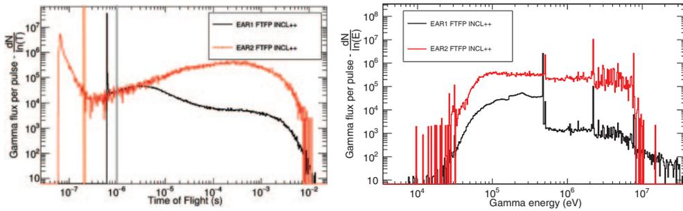
Fig. 3. – Left: Simulated  $\gamma$  flux per pulse obtained with FTFF INCL for both experimental as a function of the arrival time. The division between the prompt and delayed components is shown in grey (EAR1) and orange (EAR2). Right: Energy dependence of the DELAYED component of the gamma flux.
