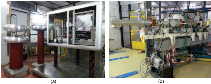
Fig. 1. – GENEPI2: (a) the deuterium ion source within the high-voltage platform (250 kV), surrounded by a Faraday cage, (b) the beam line section after acceleration transporting the deuterium beam to the target.
