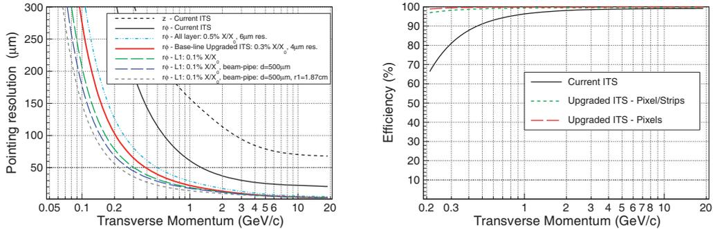
Fig. 4. – Performance of the current and upgraded ALICE ITS. Left: Pointing resolution *vs.* transverse momentum. Right: Efficiency *vs.* transverse momentum.
