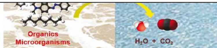
TiO<sub>2</sub> – based photocatalysts
