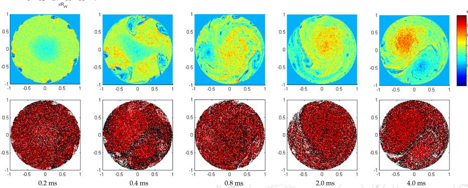
[B = 0.15 T,  $\varnothing_{trap} = 45 \text{ mm}$ , initial electron density 2.5-5 · 10<sup>6</sup>, ion fraction f = 0.3. Black: electrons, red: ions.]
