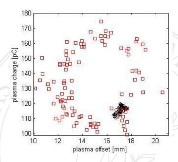
Dipole excitation 1.5 V, frequency sweep 2.3-5.2 Hz crossing the modulation frequency 4.0 Hz. No excitation (black): offset **17.1±0.5** mm. With excitation (red): offset **10.1-20.5** mm.
