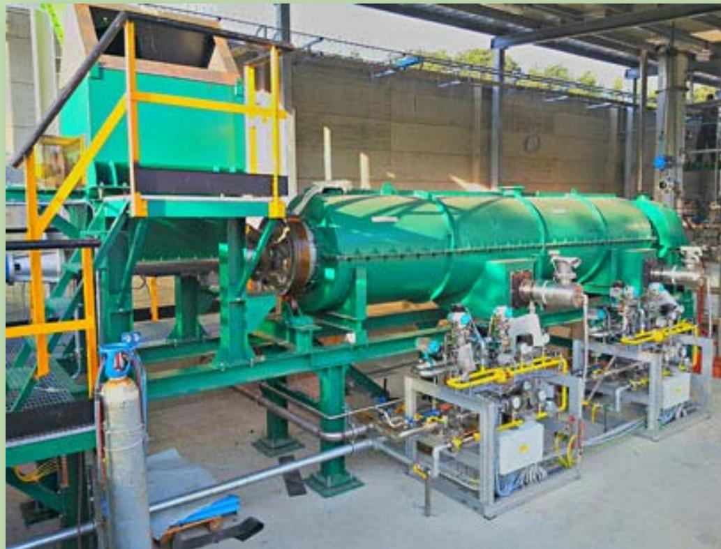
PYROLISIS → Syngas, tar, char → Mechanical Energy → Electricity (Heat)
