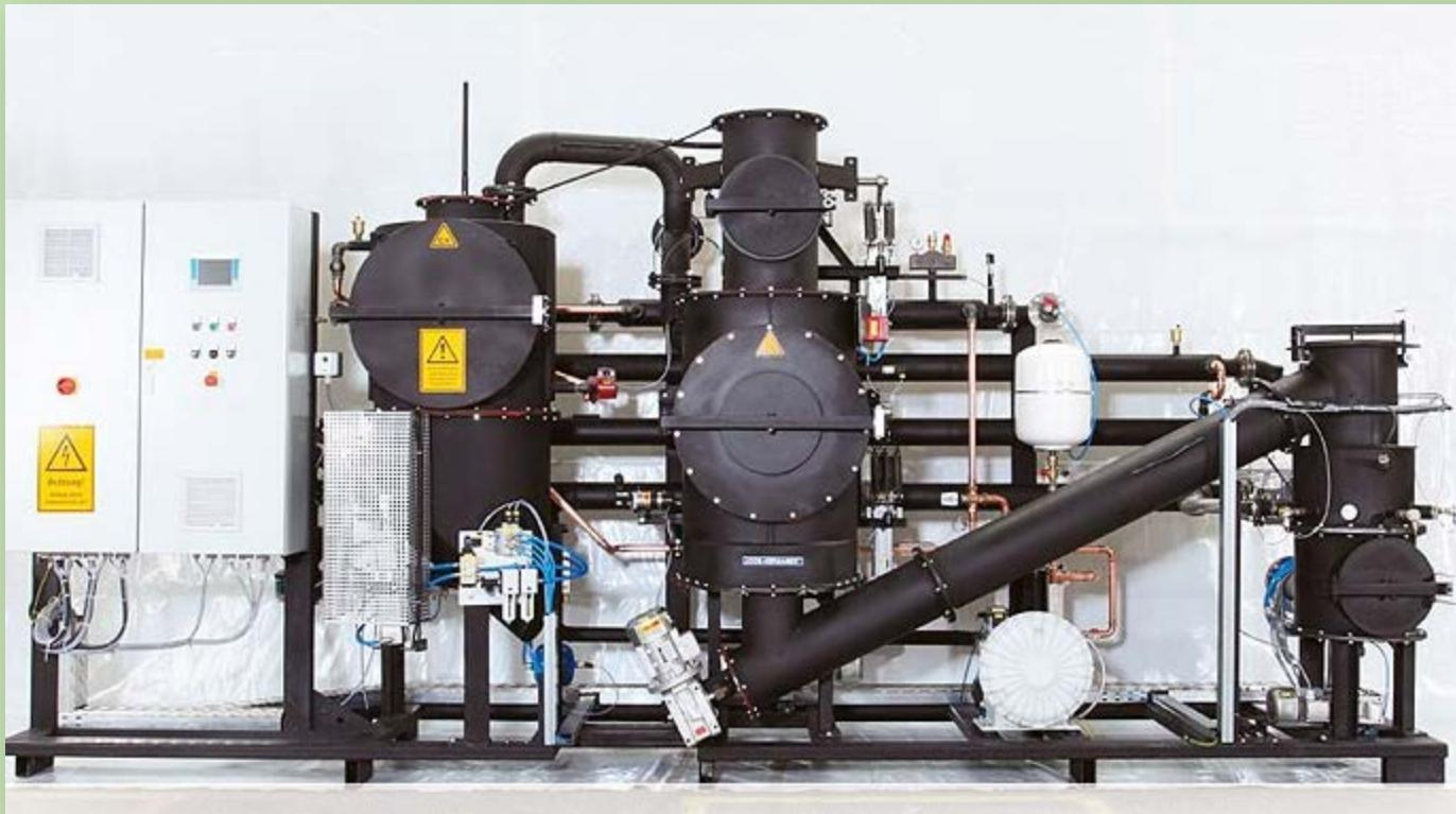
GASIFICATION → Gas → Mechanical energy → Electricity (Heat)
