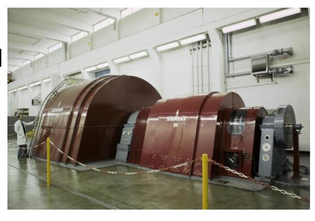
The speed of the rotors decrease by 5% during ramp-up while the generator absorbs 6 MW; during ramp-down, the stored energy flowing from the magnets, peaking at 12 MJ, reaccelerates the rotor to nominal speed
