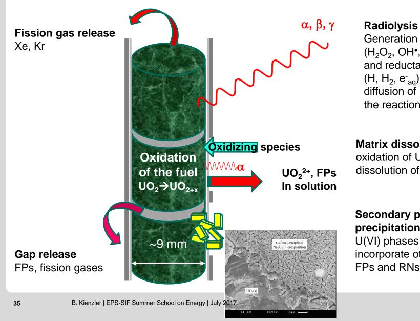
Radiolysis of water Generation of oxidants  $(H_2O_2, OH^{\bullet}, HO_2, O_2)$ and reductants  $(H, H_2, e_{aq})$ diffusion of H, H2 leaving
